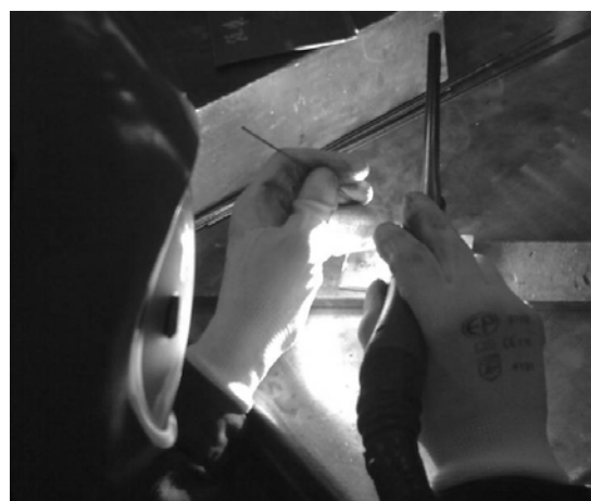
Fig. 2. Surfacing of test specimen
