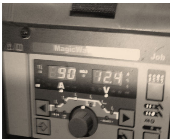
Fig. 1. Impulse equipment Fronius Magic Wave 2500 designated for TIG welding and surfacing.
