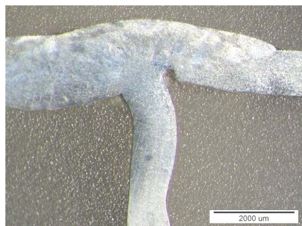
Fig. 3b. Macro structure of Spec. No2, SM. The dimensions of the weld seam measured from the image are: width B=5.42+0.03 mm; height h=0.63+0.14 mm. Thickness of the base metal d=1.04+0.02 mm
