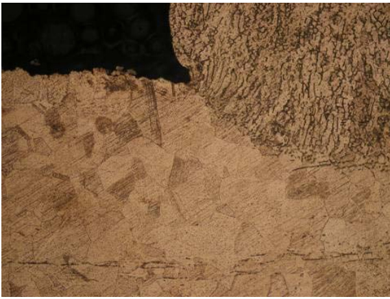
Fig. 4. Flaws in the transitions from weld seam metal to base metal, left and right end of the seam, OM
