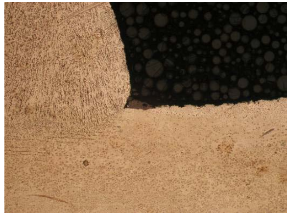
Fig. 4. Flaws in the transitions from weld seam metal to base metal, left and right end of the seam, OM
