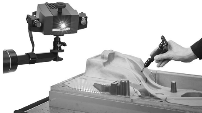
Figure 2: Optical system Atos compact scan with two cameras and blue light
