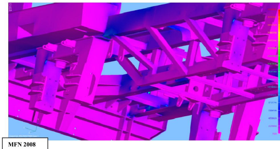
Fig. 3. Structural analysis of smash to another vehicle. Symbolic load: 1.3F_v + F_H (5g) View of the bottom center of the stand: Maximum Solid Von Mises comparative stress 388.762.432, N/m^2 .
