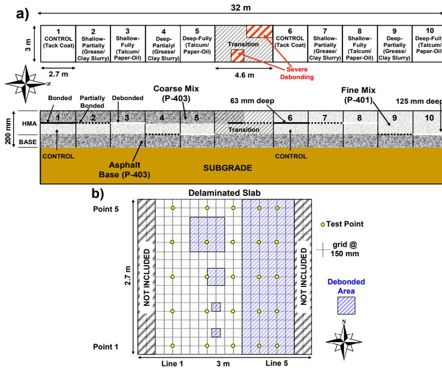
Fig. 1 Schematic of section constructed and location of test points
