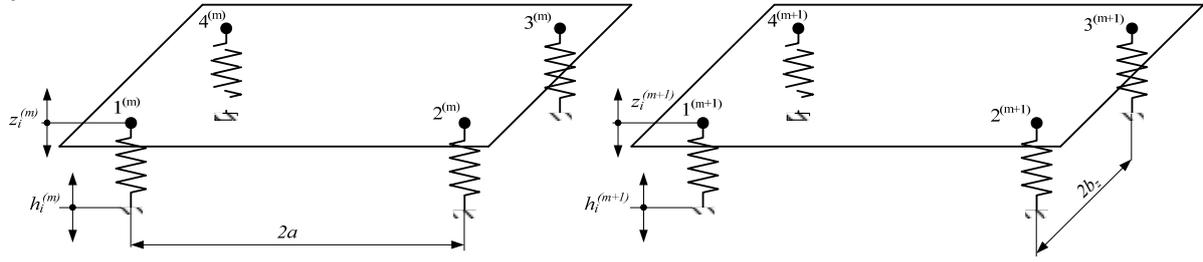
Figure 2. Model of carbody and suspension system of considered vehicle
