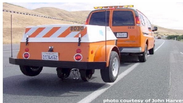
Figure 3. Dynaflect in use ( http://training.ce.washington.edu/wsdot/ )
