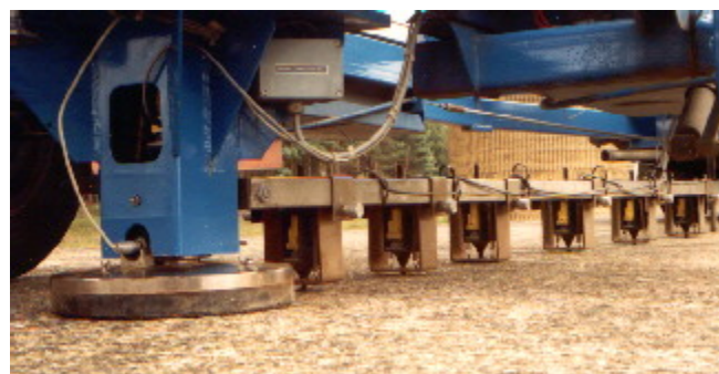
Figure 4. FWD Application ( http://training.ce.washington.edu/wsdot/ )
