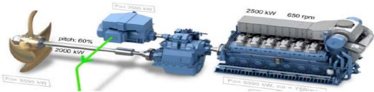
Fig. 1. Illustration of the ship's power system.
