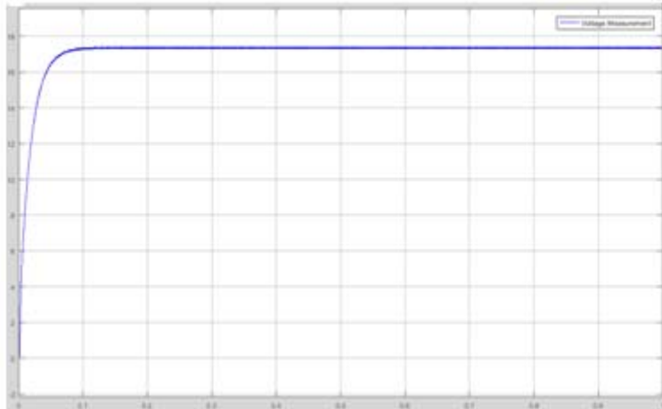
Figure 4. Oscilloscope of the output voltage waveform of the PC rectifier
