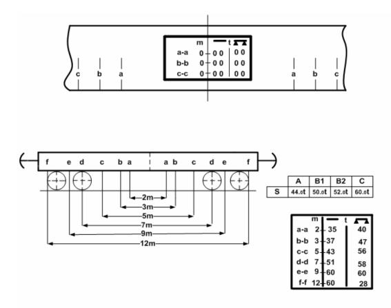
Figure 1. Marks and contents of a wagon table for freight units with leaning width  $\ge 2.00$  m
