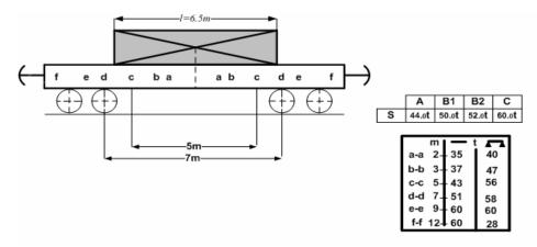
Figure 3. Elements to calculate the maximum permitted mass of a freight unit lying directly on the floor of a flat freight car between the d – d and c – c marks
