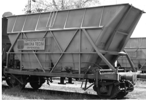
Fig. 1. Fbd wagon for transporting coal
