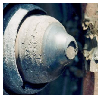
Fig. 5. Failure of axle-bearing
