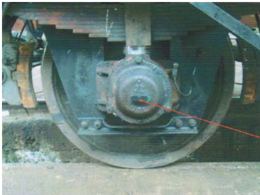
Fig. 9. Testing of transmitting sensor unit on axle-box bearing
