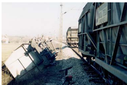
Fig. 4. Derailment of wagons for coal transportation
