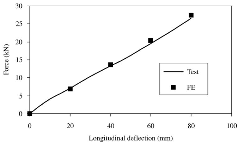
Fig. 4. Stiffness comparisons between the test and the FE simulation
