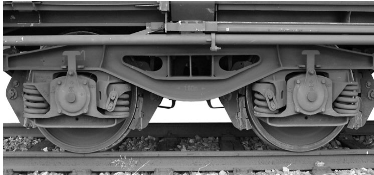
Fig. 9. Suspension of freight bogie Y25
