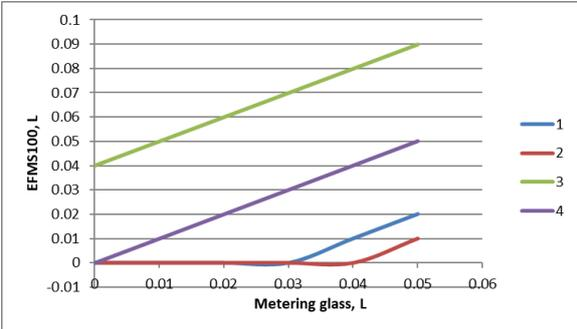
**Fig.4 Fuel flow metering characteristic at Partial load mode with low rpm**
