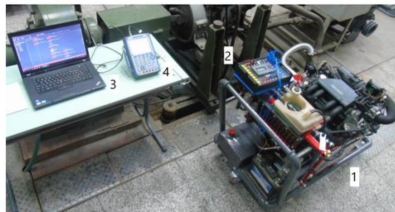
**Fig.2. Test bench SKAD-1: 1-engine; 2-controller MI0245 [8]; 3-computer equipment; 4-measuring equipment**
