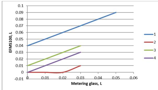
**Fig.5 Fuel flow metering characteristic at Partial load mode with high rpm**
