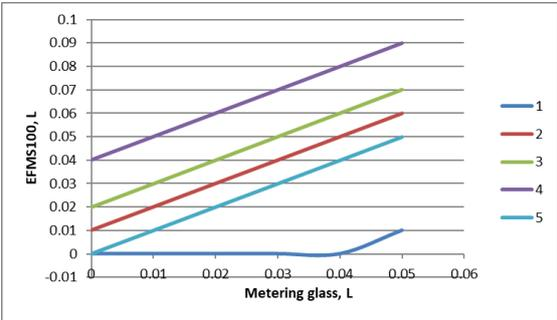
**Fig.3 Fuel flow metering characteristic at Idle mode: 1,2,3,4,5-number of experiments**
