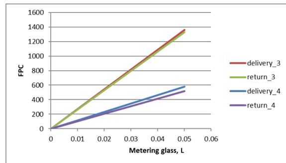
**Fig.8 Calibration characteristic at Partial load mode at high rpm and Full load mode**
