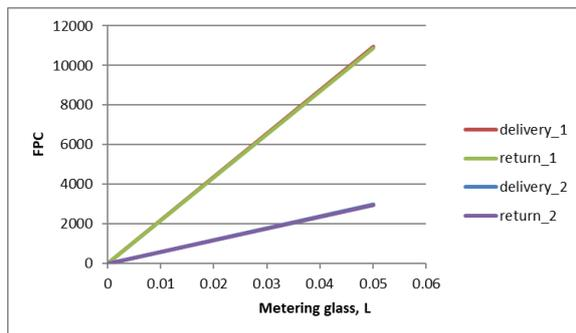
**Fig.7 Calibration characteristic at Idle mode and Partial load mode at low rpm**
