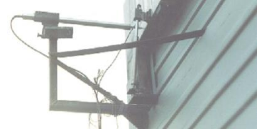
Figure 2: The testing of roof movement (Hccrrss-z)
