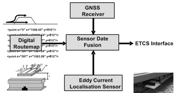
Fig.5. Multi sensor system for autarkic localization
