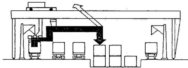
*Fig. 1 The second generation of gantry cranes for container handling [3]*
