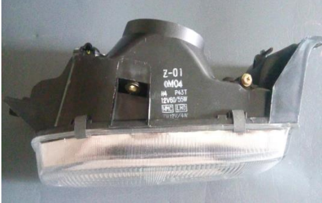
Figure 2. Dipped-beam headlamps without Indication of the initial downward inclination
