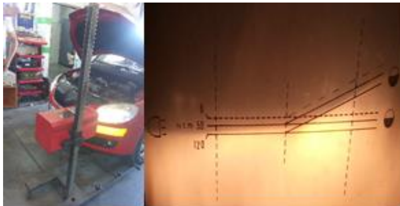
Figure 9. Measurement the direction of the headlamps by device with fixed screen.
