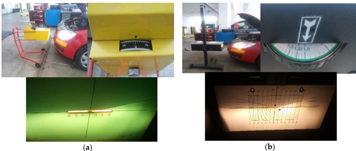
Figure 8. (a) Measurement the direction of the headlamps by device with adjustable screen which scale is in cm/10m; (b) Measurement the direction of the headlamps by device with adjustable screen which scale is in %.
