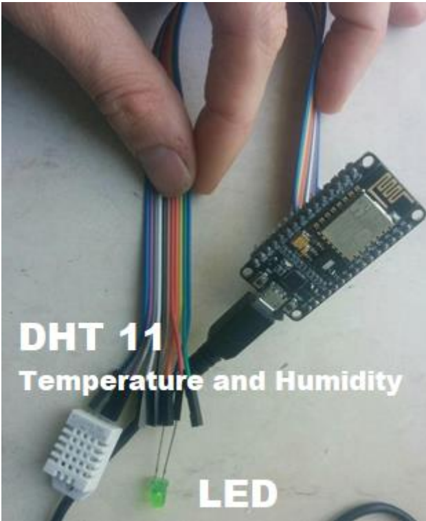
Figure.1 Experimental setup of Node MCU esp8266 built-in system
