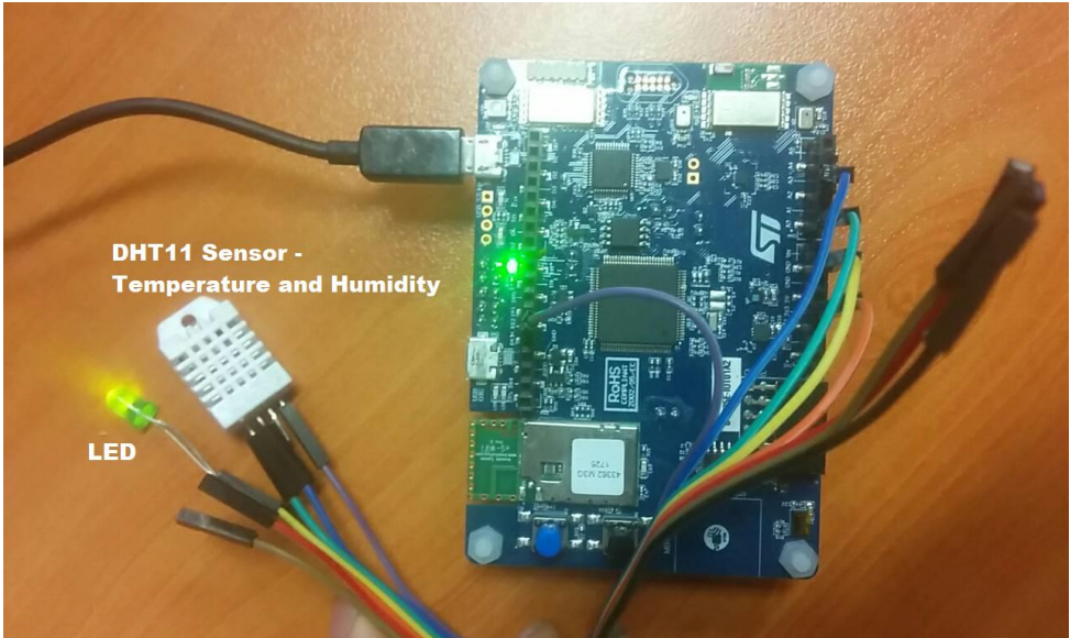
Figure.2 Experimental setup of STM32L4 discovery IoT node
