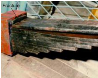
Figure 8. The fracture of main leaf of LS 1
