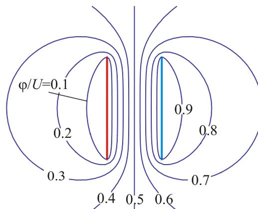
**Fig.4 Equipotential lines for parallel plate capacitor with air-filled dielectric.**
