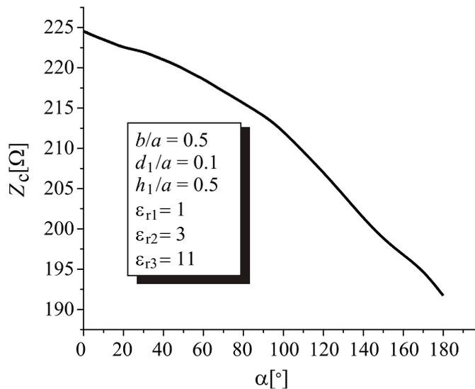
**Fig.7 Characteristic impedance distribution versus boundary surface position.**
