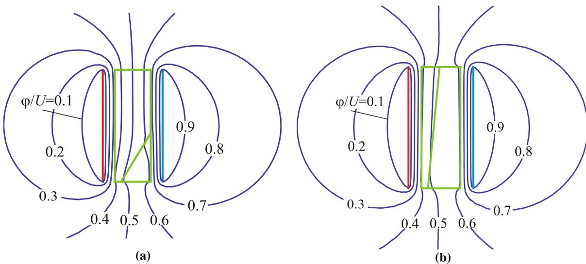
**Fig.5 Equipotential lines for: (a)  $\alpha = 60^\circ$  and (b)  $\alpha = 85^\circ$ .**
