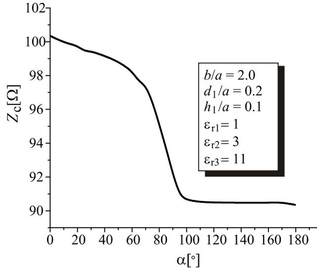
**Fig.6 Characteristic impedance distribution versus boundary surface position.**
