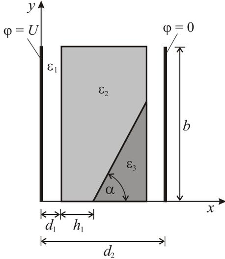
**Fig.1 Parallel plate capacitor with angled boundary surface.**
