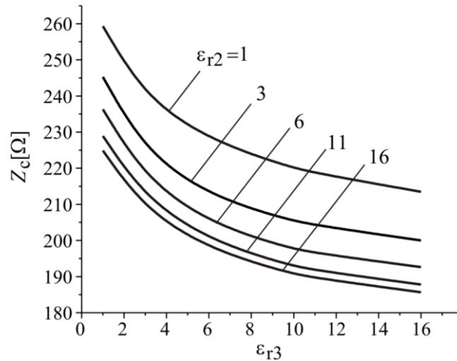
**Fig.8** Characteristic impedance distribution versus different permittivities  $\epsilon_{r2}$  and  $\epsilon_{r3}$ .
