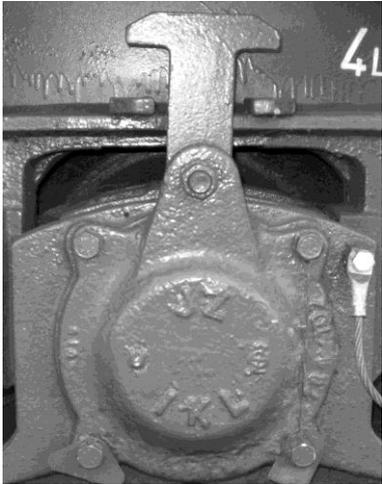
Fig. 4 Stroke limiter
