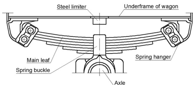
Fig. 2 Connection of leaf spring and underframe
