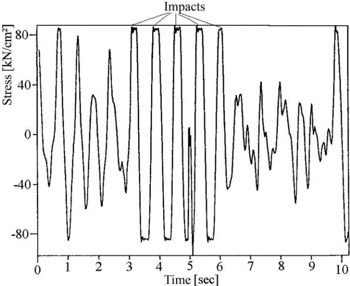
Fig. 5 Diagrams of change of stress on the elements of suspension during the time
