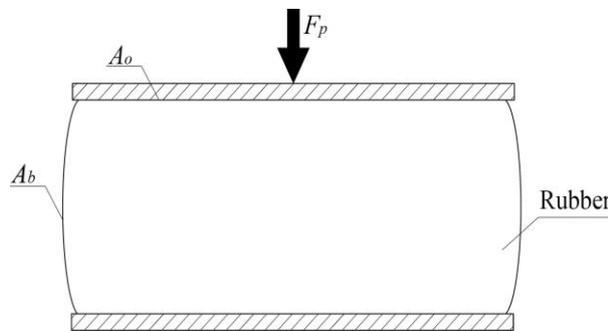
Fig. 8 The reinforced rubber elastic element
