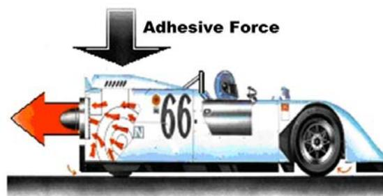
**Fig.7B. The path of the air thrown out by the turbines.**
