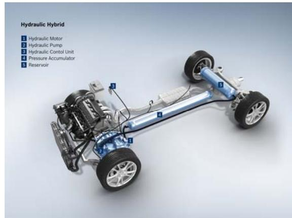
Fig.3B. The prototype of Bosch.
