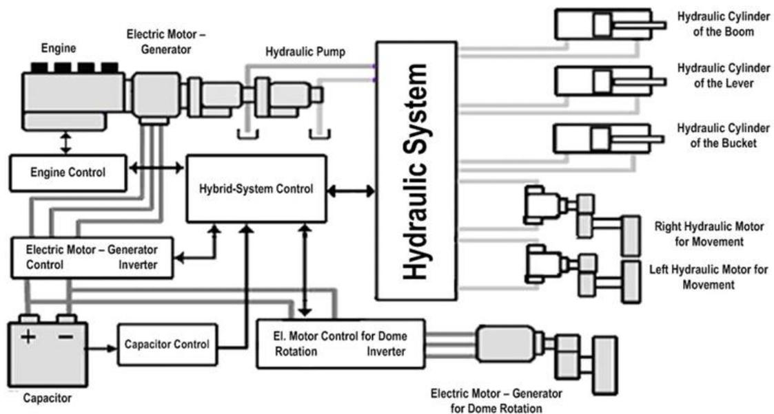
Fig.1. Scheme of the latest generation of hybrid excavators.
