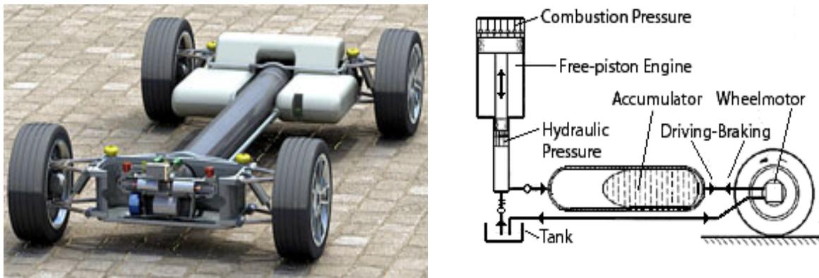
Fig.2. Hybrid hydraulic car of INGOCAR.
