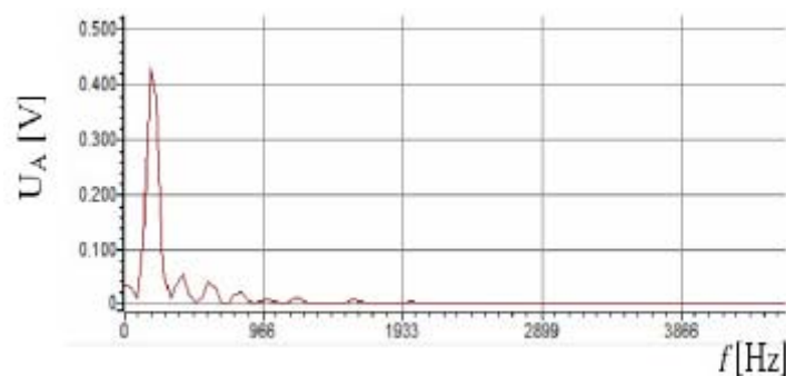
Fig. 5. Amplitude spectrum of triangul waveform.
