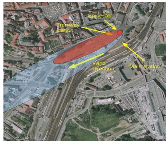
Picture 4. The contamination extent by mortal and injuring chlorine concentration
