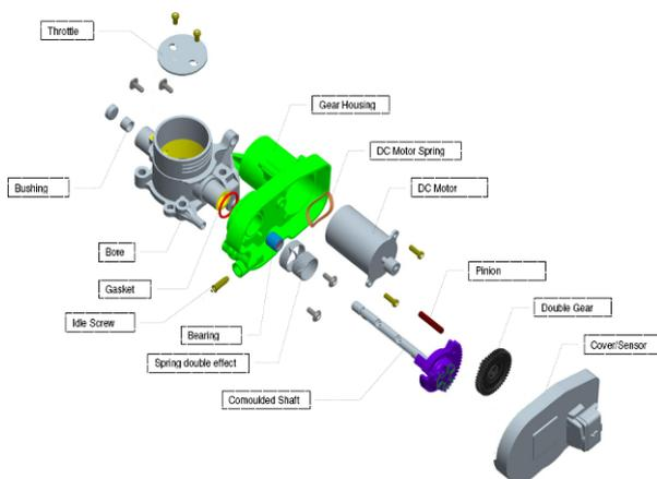
**Figure 3. Exploded view of a throttle body**
