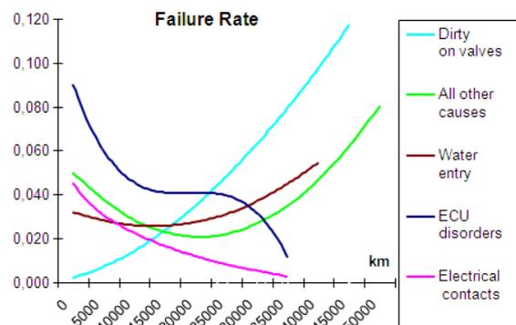
**Fig. 4. Failure rates from in-field data**
