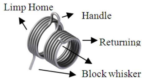
Fig. 8: Double torsion spring with its two parts of “Limp Home” and “Returning”
