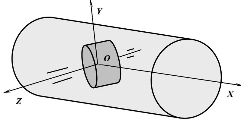
**Figure 1.** Two bodies - a lifting and lifted axi-symmetric rotor.
